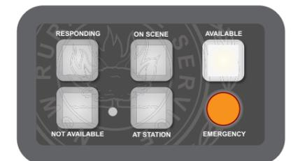
When the keypad has been idle for 5 minutes, the keypad status buttons will **GLow WHITE**.
