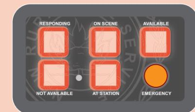
The keypad buttons **FLASH RED** when the keypad can't communicate with the radio. **No status updates can be sent at this time.**
