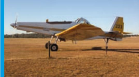
Turbine Dromader uses AVGAS fuel at the rate of 250 litres per hour, has a cruising speed of 240kph and carries 2,500 litres.
