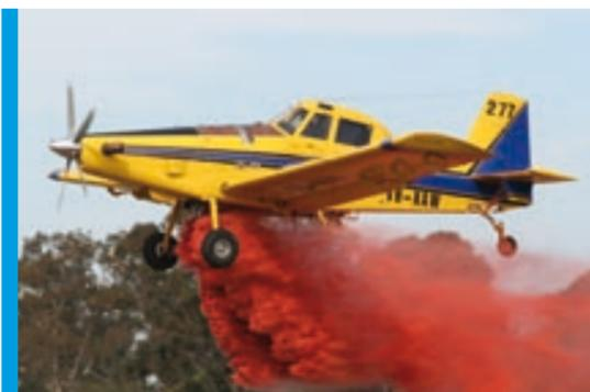
Air Tractor AT 802 uses Jet A1 fuel at the rate of 280 litres per hour, has a cruising speed of 280kph and carries 3,200 litres.
