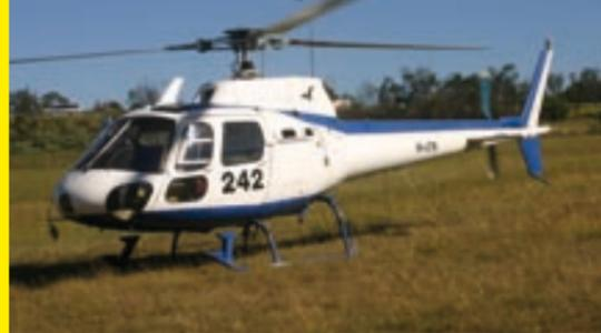
Squirrel AS350 with one engine and 3 blades, uses Jet A1 fuel at the rate of 170 litres per hour, has a cruising speed of 224kph and carries 680 litres.
