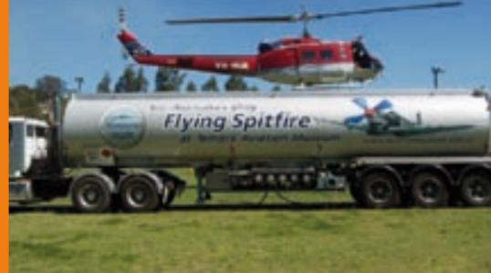
Bell 204 Restricted Category, with one engine and two blades, uses Jet A1 fuel at the rate of 320 litres per hour, has a cruising speed of 200kph and carries 1,500 litres.
