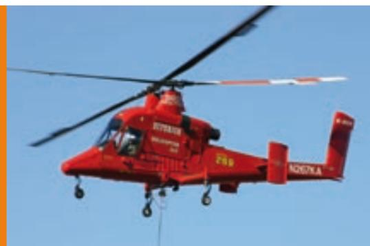
Kaman K-Max with single engine driving two side by side intermeshing, counter rotating blades, uses Jet A1 fuel at the rate of 253 litres per hour, has a maximum speed of 185kph and carries 3,000 litres.
