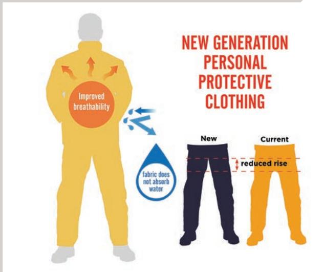
The upgrade and review of Personal Protective Clothing (PPC) has reached another milestone. In October 2016 the latest prototypes underwent testing at the University of Alberta in Canada. Under laboratory conditions the PPC was tested for its capacity to protect a firefighter in the event of a flashover. The garments underwent temperatures of 800-900 degrees Celsius for four seconds. The garments emerged from the test meeting all the standards and being comparable with the current PPC.
