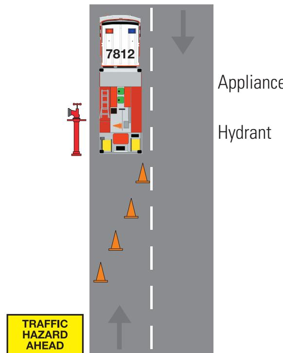
Installation or maintenance of hydrant markers on two lane road with speed limit 70 kph or less
